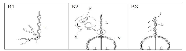
Step B1: By measuring, determine the correct number of links needed for proper hanging height. Using the chain pliers, disconnect and discard the remaining chain.
