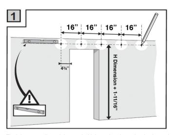
Find the centerline of the track. Using a level, mark a horizontal line twice the door width long. Mark the bracket screw locations into the wall blocking. Attach the wall portion of the brackets as shown.
