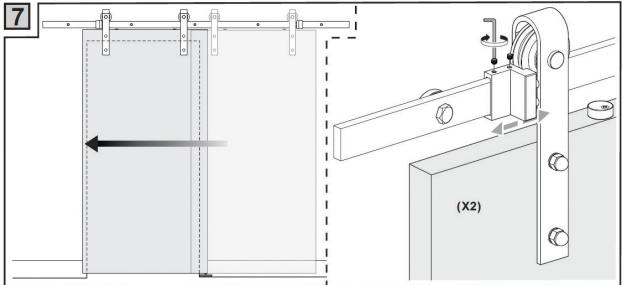
Adjust the door stops accordingly using the provided 2.5mm Allen key.
