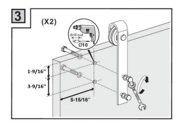
Drill out holes in the door using a 10mm routing drill bit as pictured. The bottom of the door should be routed at this time in order to accept the floor guide.
