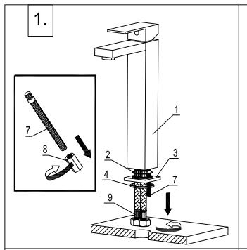
1. Make a hole of Ø32~Ø35(Ø1 1/4"~Ø1 3/8") on the basin deck, screw off the lock nut (8) from the long rod (7), screw the long rod and water supply hose to the body(1),and tighten with wrench. Put whole faucet into the hole with the washer(2), base (3) and gasket(4) between basin deck and faucet.
