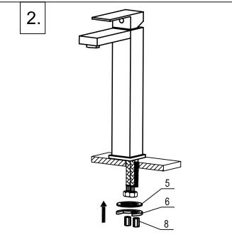
2. Fixing the faucet from downside the basin deck, with rubber washer(5), metal gasket(6) and lock nut  $\ (8)$  .
