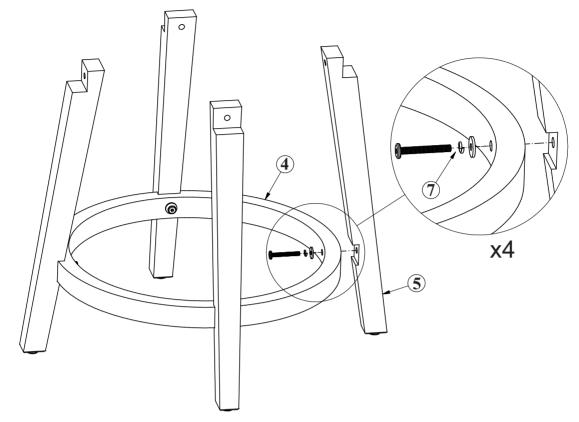
Attach each leg (5) to bottom frame (4). Insert each individual set of hardware as per picture show. **Do not tight up any hardware completely.**
