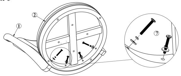
Insert 4 sets hardware first, then tighten together after alignment is done
