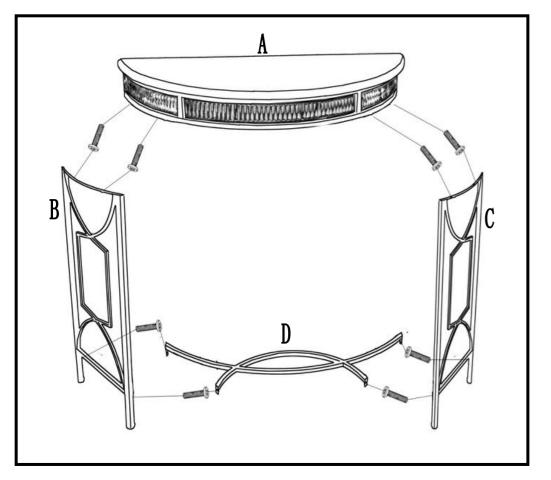
Attach all parts together, use Allen Key to tighten all bolts.
