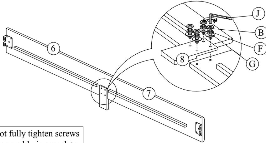
Do not fully tighten screws until assembly is complete and the bed is level.
