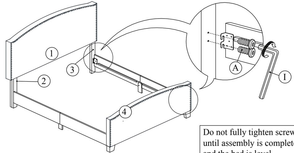
Do not fully tighten screws until assembly is complete and the bed is level.
