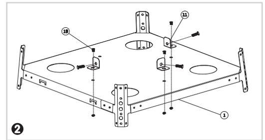
**3** Assemble the lower frame. Remove the **Screws 18** pre-assembled in their respective eyelets. Align the eyelets at the bottom of one of the **Lower Supports 11** with the eyelets at the corners of the **Bottom Plate** and **Middle Plate** using the **Screws** removed earlier.
