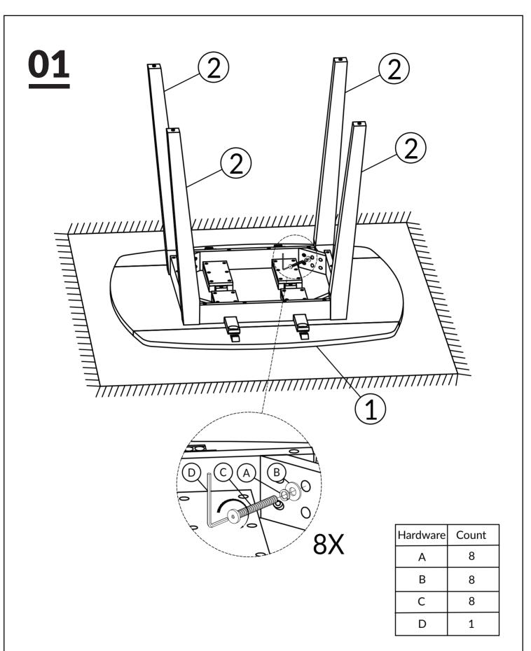
TIGHTEN BOLT COMPLETELY.
