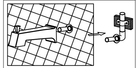
11. Insert the spout to the pipe which outside the wall, then tighten the screw.
