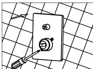
6. Lock the deck plate into the body and cling to the wall, then tighten the screw.
