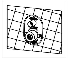
4. Please cut the size of the tile hole according to the size and shape of the protected cover ( about 5mm bigger than the protected cover from each side ). And please put the tile outside the wooden wall ( please noted that we keep the same central point for the tile hole with the protected cover ) .
