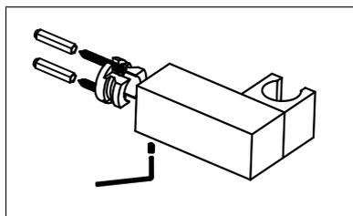
10. Loosen the hex screw of the connector, take out the nut to insert with 2 screws into the hole in the wall. Insert the connector and tighten the hex screw .
