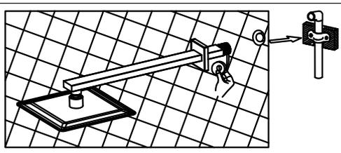
9. Install the shower arm, shower head and flange to the fitting. (stick to the wall) . Tighten the showerhead to the shower arm with the pipe tape. (Make sure the pipe tape with clockwise direction) .
