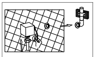
8. Insert the spout to the pipe which outside the wall, then tighten the screw.
