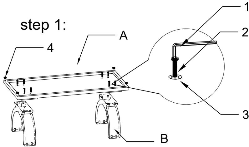
Fit the adjust legs (4) to bottom base, Connect Stainless steel pillar (B) with Stainless steel base (A) by Screw (2) (M8\*40), tighter, one by one
