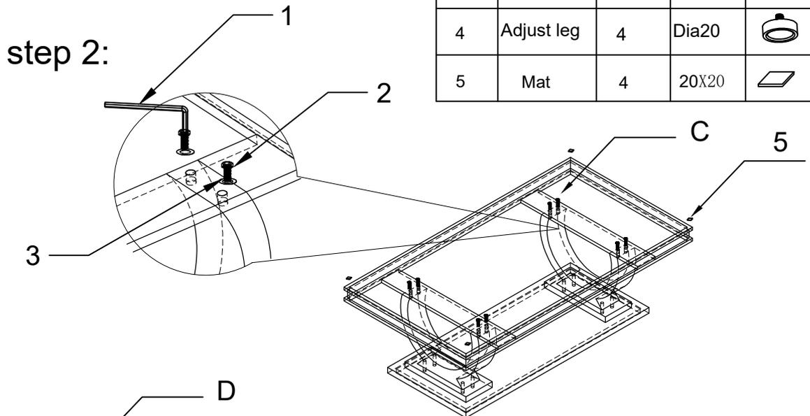
Place the Table top (C) on the stainless steel pillar (B) as shown. Then, install the stainless steel pillar (B) to the table top (C) from the bottom by the screw (2) (M8\*50)
