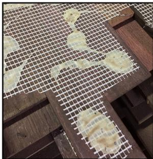
**Note:** The glue & mesh backing is to aid in positioning the panels during installation only. It is not intended to be a structural support of any kind. Should any pieces pull away from the mesh backing prior to installation, simply install the panel as normal, then reinsert the loose piece and nail individually.
