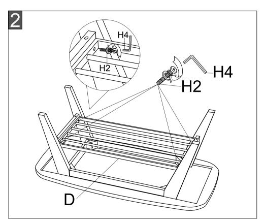
Step 2: Attach the metal shelf (D) to the assembled connecting bars by using the Allen key (H4) to lock with 4\*Allen bolts (H2), as picture. Straighten up the assembled product, Assembly is completed.
