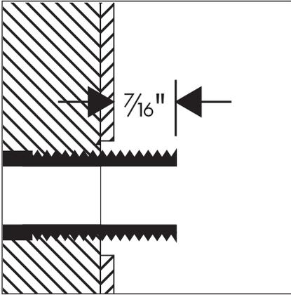
This unit requires a 1/2" NPT male nipple, extending 7/16" outside the surface of the finished wall.
