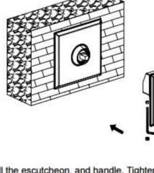
Install the escutcheon, and handle. Tighten the set screw with an Allen wrench to secure.
