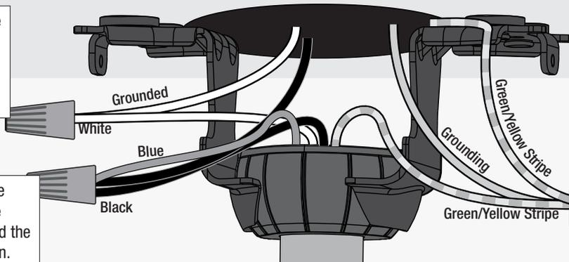
Connect the three grounding wires (green, green/yellow stripe, or bare copper) coming from the ceiling, downrod, and hanging bracket.
