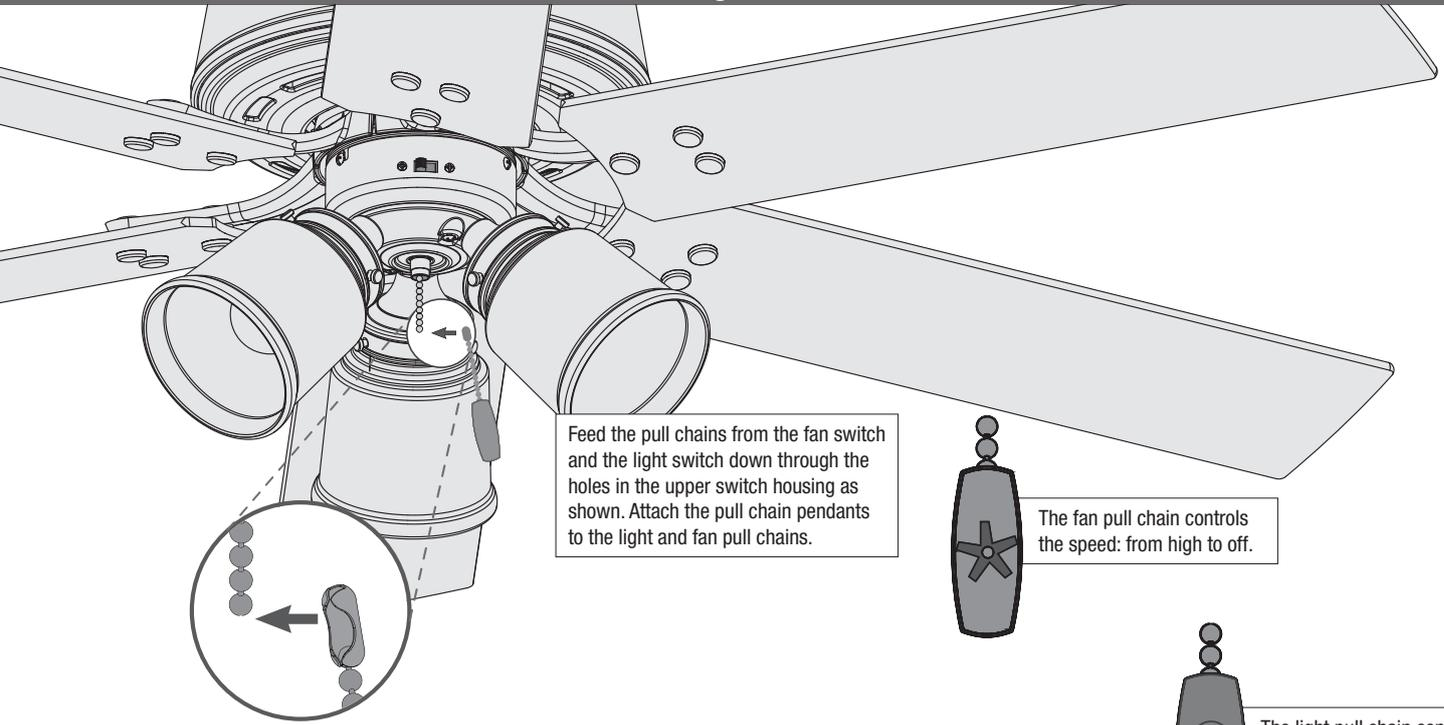
Feed the pull chains from the fan switch and the light switch down through the holes in the upper switch housing as shown. Attach the pull chain pendants to the light and fan pull chains.
