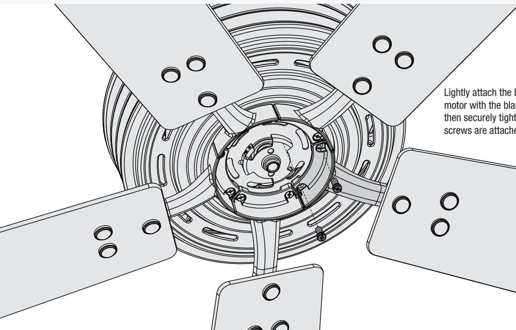
Lightly attach the blade arms to the motor with the blade arm screws, then securely tighten after both screws are attached.
