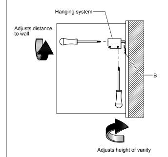
Secure cabinet (A) to the wall using long screws (D). Make sure to drive screws (B) into re-enforced area of the wall.
