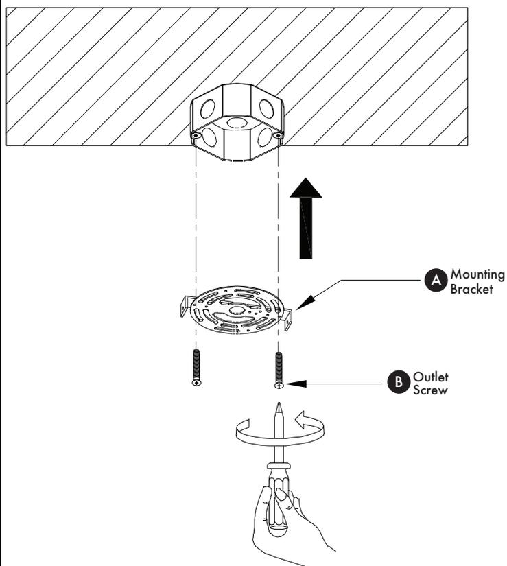
**Secure mounting bracket (A) with outlet screws (B).**
