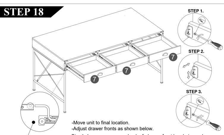
The drawer rail pulley is put into the table guide from the top
