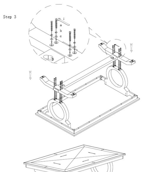
STEP 3: Assemble with flat washer [c], lock washer [b], bolt [a] in the vertical direction.
