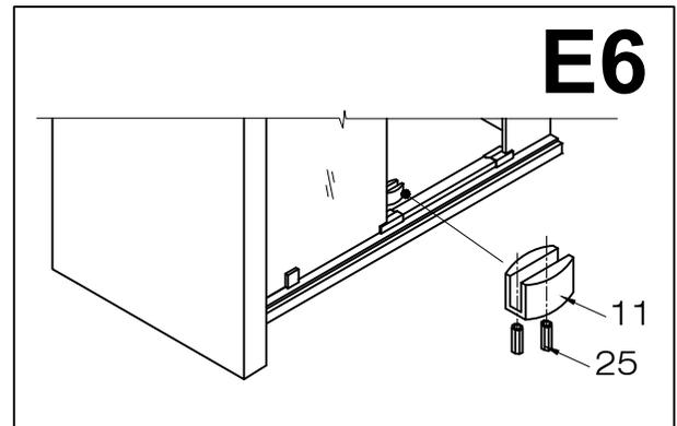
7. Screw the door guide to the floor with 1 1/8" screws (#21).
