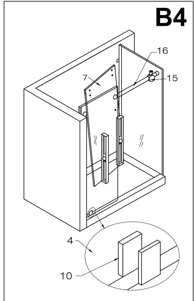
5. Remove the big front fixed panel from the position in the opening. Unscrew and detach the fixed panel bottom clip (#10) from the big front fixed panel and place it where you marked the floor. Mark a hole on the floor for the mounting screw.
