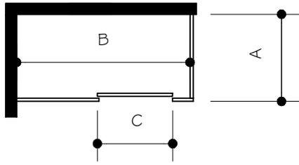
DIMENSIONS 'A' AND 'B' INCLUDE GLASS, SEAL STRIPS AND HARDWARE
