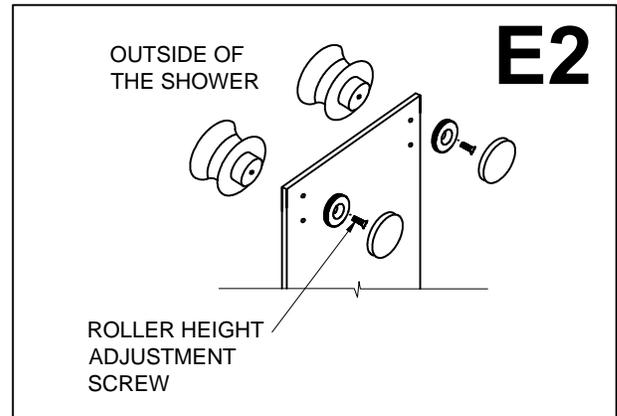
3. Place the two top rollers and the door panel (#7) assembly onto the structural rail (#16).
