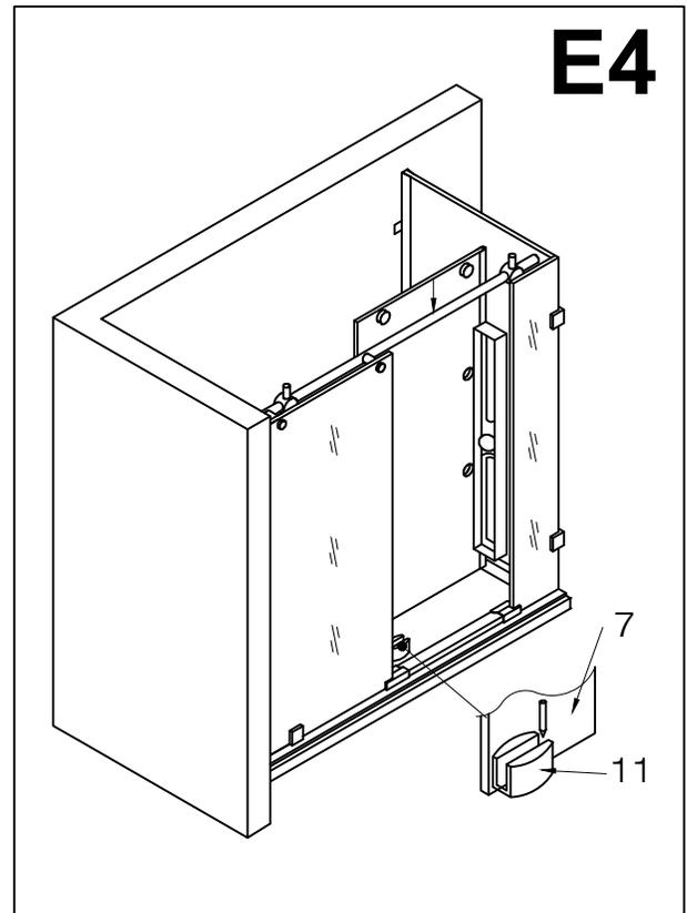
5. Remove the door from the structural rail. Mark holes on the floor for the mounting screws.
