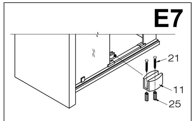
8. Place the door back on the structural rail. Screw the bottom rollers (#3) to the door. Follow step E2.
