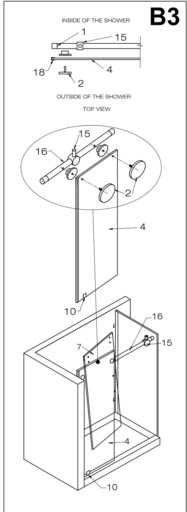
4. Make sure the front fixed panel is level and mark the fixed panel bottom clip (#10) location on the floor.
