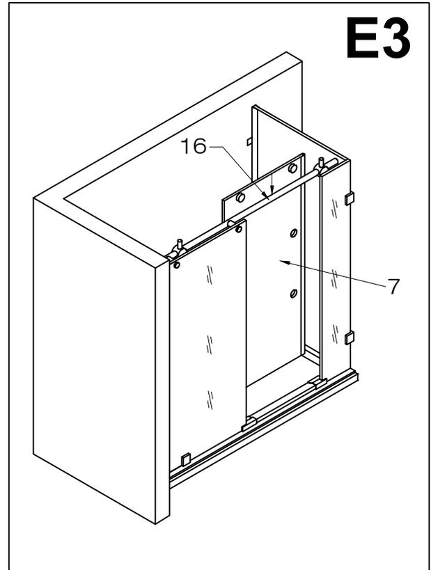
4. Align the door guide (#11) onto the door. Use a level to make sure the door is straight. Mark the location of the bottom door guide on the floor.
