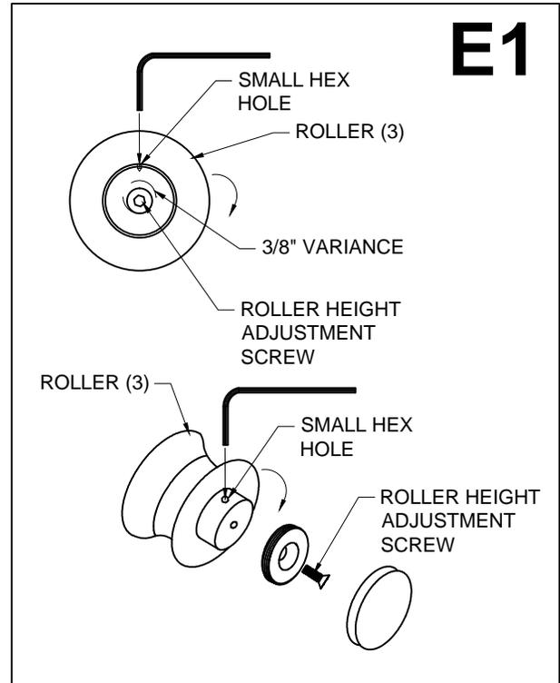
2. Use the provided allen key to unscrew the adjustment screw and dismantle the roller. Place the screw through door panel top holes and attach the two top rollers onto the door panel (#7).
