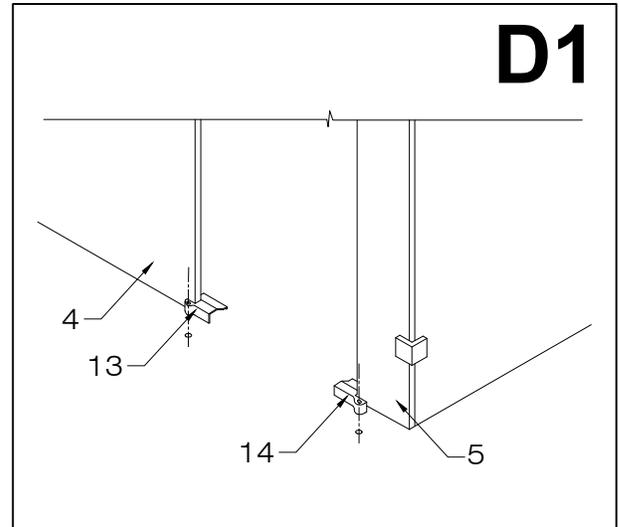
2. Remove the threshold clips (#13 and #14). Drill holes into the respective marks and put plastic anchors (#25) in them. **⚠ Not necessary if installing into studs. Studs are the preferred means of installation, anchors can pull out of the wall causing property damage and bodily harm.**
