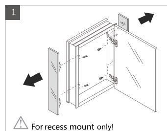
Carefully remove side mirror panels for recess mount installation.
