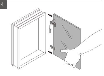
Take off the door(s) carefully and lay it down on a safe area.
