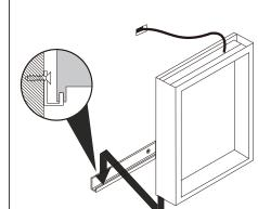
With assistance, to rest the cabinet on the Insert top mounting bracket into the top mounting bracket and hold in place.
