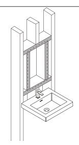
Frame the opening for the cabinet based on the measurements.
