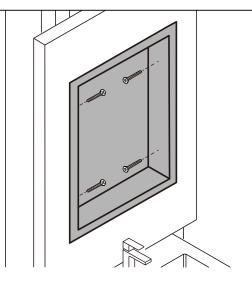
Affix using hardware screws into the studs.
