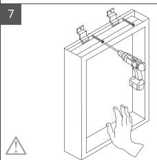
Top mounting brackets must be attached to furring strip/channel or wall studs.
