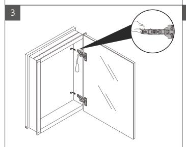
While supporting the door release(the lever under the hinge arm), slide the door off the frame.
