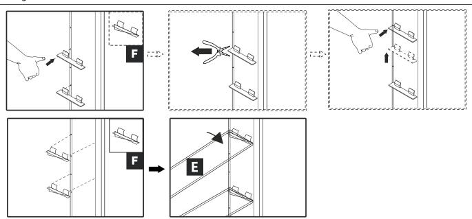
1.Insert clear snap in shelf clips (F) into holes on the sides of the cabinet cabinet.
