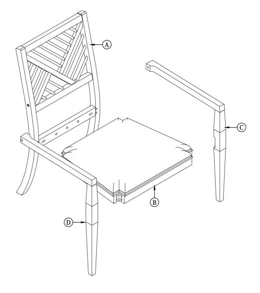
Note: Do not tighten bolt before all component assembly
