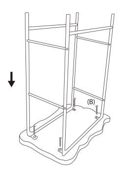
Put the wood boards on the metal frame and secure them by the screws B.
