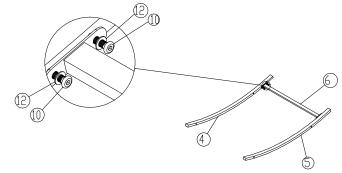
Assemble metal tube G to legs D and E using spring washers L, bolt J and caps M.
