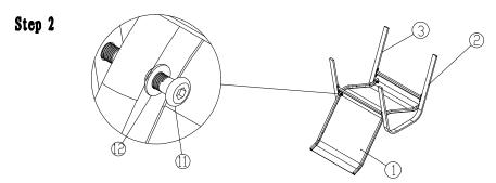
Assemble the back frame A with textilene fabric to the side bars C and B using washers L, bolts K and caps M. Please DO NOT over-tighten the bolts!
