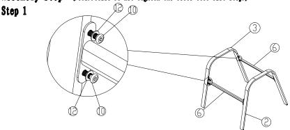
Assemble the metal tubes F to side bars C (Right) and B (Left) using washers L, bolts J and caps M.
