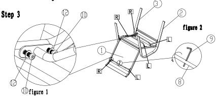
Assemble adjustable bars H to the back frame A using washers L, bolts J and cap M shown in figure 1. (Adjust turning tube in middle of bar H to adjust length to fit) Then put the plastic tube N onto the adjustable bars H to cover the exposed groove shown in figure 3.
