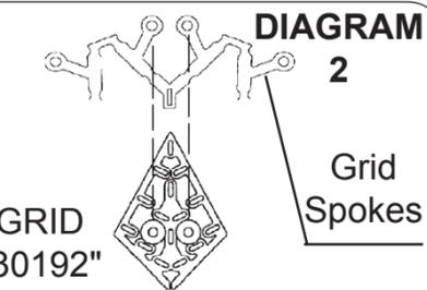
**Installation of Grid "30192":** Attach (8) Grids "30192" with two thumb nuts per grid (already screwed onto grid) to 8 ring. Diagram 2. (See page 5 for location on frame)
