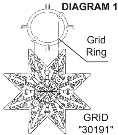
**Installation of Grid "30191":** Attach (1) Grid "30191" (with finial attached) with two thumb nuts (already screwed onto grid) to 9 ring. Diagram 1. (See page 5 for location on frame)
