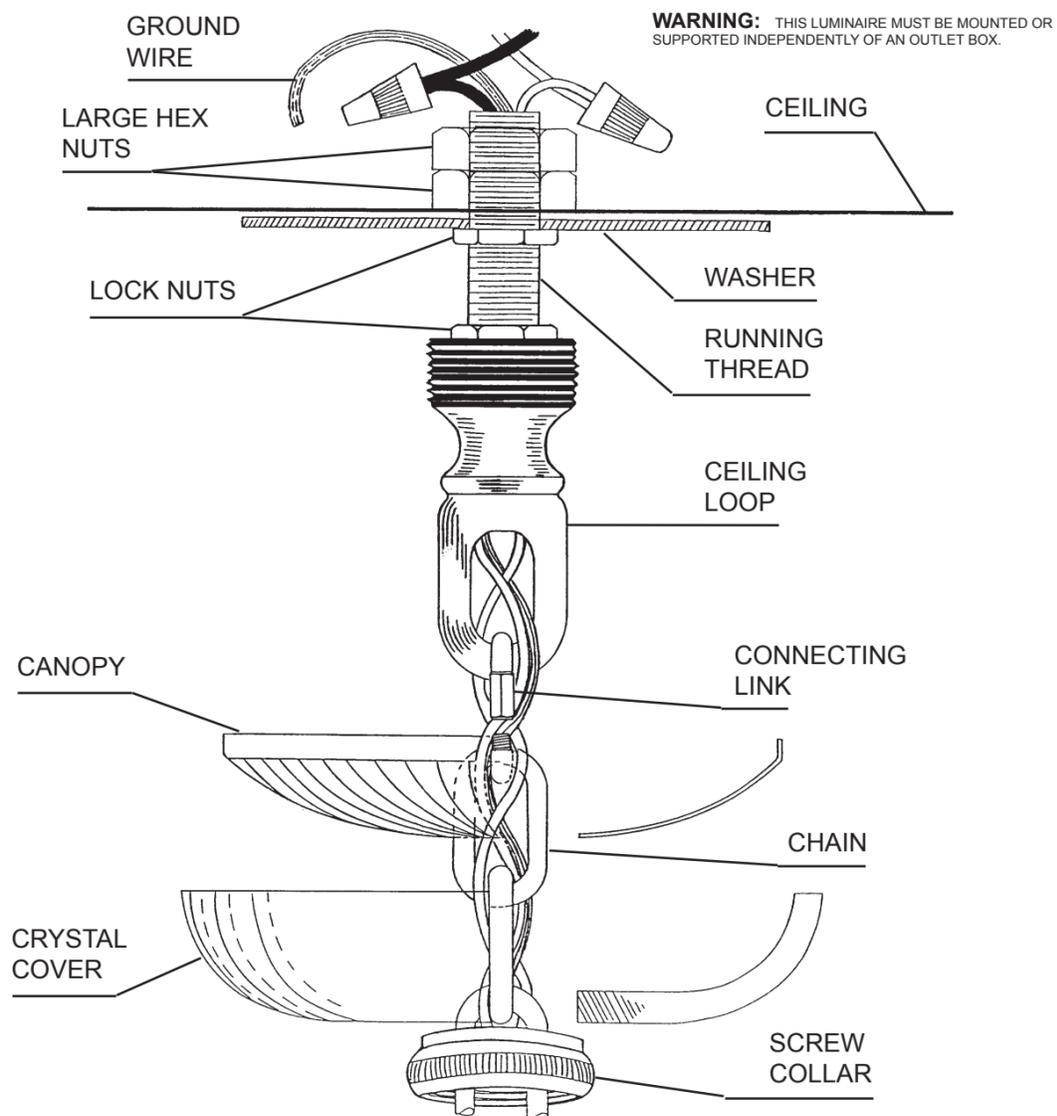
**WARNING:** THIS LUMINAIRE MUST BE MOUNTED OR SUPPORTED INDEPENDENTLY OF AN OUTLET BOX.
