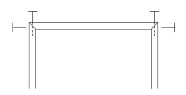
Drill holes with a diameter of  $5/64 \times 6/64$ ". Tighten with  $1/4 \times 2$ " screws.
