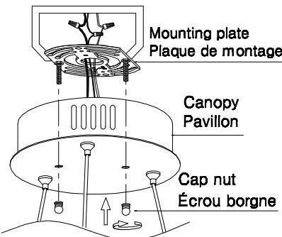
Install the canopy to mounting plate with 2 cap nuts provided.
