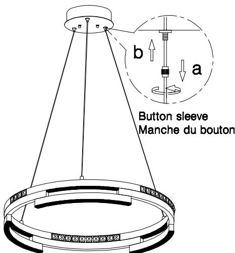
Before installation to ceiling, adjust fixtures to desired length by pushing wire up into canopy, then coiling up excess wire, minor adjustment can be made after installation. To lower or lengthen wire, depress button sleeve located where wire comes out of canopy.
