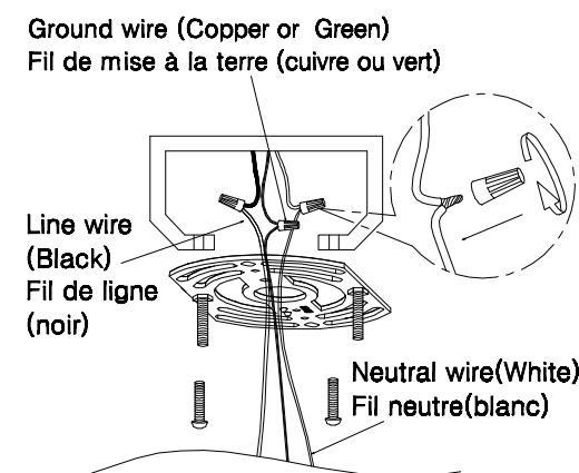
Connect the GROUND WIRE from junction box to GROUND (or GREEN) with from fixture by using a wire nut. (Or attach them to the mounting plate with a green ground screw) Connect the NEUTRAL WIRE from junction box to NEUTRAL (or WHITE) wire from fixture with a wire nut. Connect the LINE WIRE from junction box to LINE (or BLACK) wire from fixture with a wire nut.
