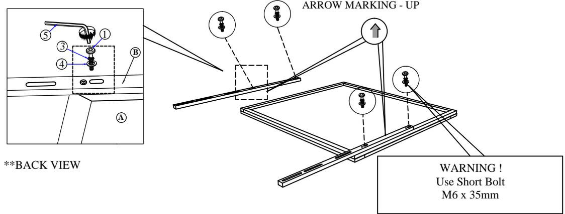
**STEP 3 :** Place mirror (A) on top of dresser (C). Align & fasten mirror support (B) to the back of dresser (C) using JCBC bolt (2) , spring washer (3) & flat washer (4) **THEN FULLY TIGHTEN ALL THE BOLTS AT STEP 2 & 3 WITH ALLEN KEY ( 5).**
