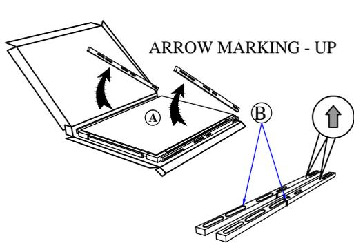
**STEP 2 :** Align & fasten mirror support (B) to the back of mirror (A) using short JCBC bolt(1),spring washer (3) & flat washer (4). **DO NOT FULLY TIGHTEN AT THIS STEP.**
