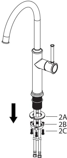
Remove the mounting screws (2C), mounting nut (2B), and rubber & metal washer (2A) from the mounting pipe
