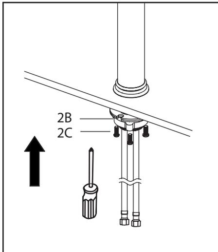
Adjust direction of faucet body (1) so that handle is on right side of faucet. Tighten mounting nut (2B) until snug. Tighten mounting screws (2C) to nut with Phillips screwdriver until snug
