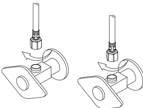
Attach waterlines(3) to angle stops and tighten until snug. Turn on angles stops and check for leaks **(DO NOT TURN FAUCET ON)**
