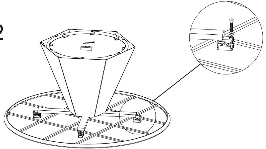
Place the base over the table top fitting the assembly brackets using 1" bolts and flat washers. Confirm legs are attached at correct angle and fully tighten all bolts.
