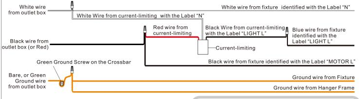
Warning: If you would like to use wall switch to control the light and fan, please refer to the switch installation instructions.
