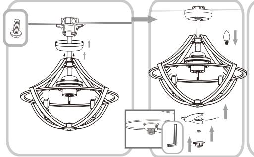
Lift Ceiling Canopy to the Hanger Frame and attach screws to lock canopy in place on the Hanger Frame
