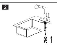
From below, put RUBBER GASKET, STAINLESS STAIN WASHER, LOCKNUT and SCREWS through THREADED SHANK in order.
