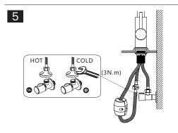
Connect HOT&COLD WATER PIPES to valves respectively.
