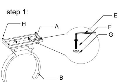
Fit the adjust legs (4) to bottom base, Connect Stainless steel pillar (B) with Stainless steel base (A) by Screw (2) (M8\*60),tighter, one by one
