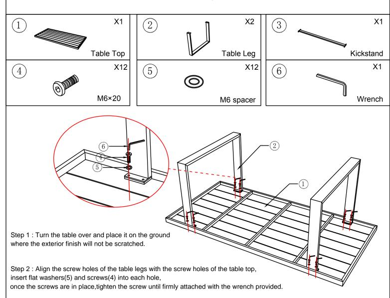
Step 3: Insert the flat washer (5) and screw (4) into each hole, and then install the Kickstand.
