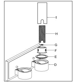
Step.3: Put the round glasses (E) into the cups (D). Put the bulbs (G) onto the sockets which inside the cups (D).
