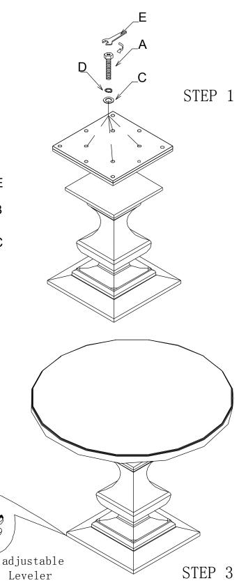
Adjust leveler if needed to level case on uneven floor.
