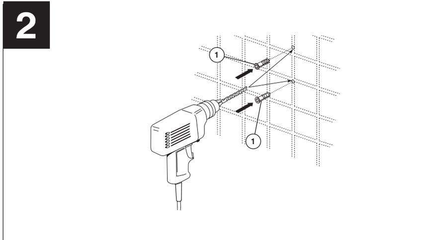
**NOTE:** If possible, it is best to mount at least one end of your towel bar into a wall stud. Try to locate a wall stud with a stud finder or by tapping on the wall. Place mounting bracket (1) in the desired location. Ensure the mounting bracket is level; then, mark the position of the holes (2) on the wall. Repeat for 2nd mounting bracket, spaced as noted above.
