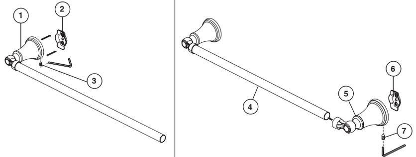
Position body (1) over mounting bracket (2) and tighten set screw (3). (Set screw should be on the bottom of body.) Place one end of the towel bar (4) into the second body (5), and place the other end of the bar into the first body (1). Slide the second body over the other mounting bracket (6) and tighten set screw (7).
