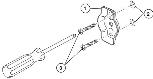
With the mounting bracket (1) oriented as shown, place it over the installed anchors (2) and screws (3). Repeat for second mounting bracket.
