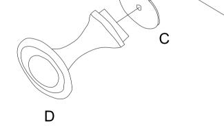
Do not use screwdriver to attach handle, tighten by hand with light pressure on screw making sure plastic washer is between handle and mirror
