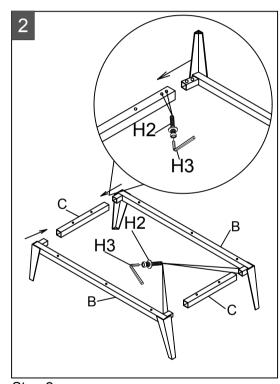
Step 2: Attach 2\*Connecting bars (C) to the both legs (B), using Allen Key (H3) to lock with 8\*Allen bolts (H2). As picture.
