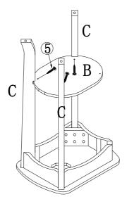
Insert Bottom Panel (B) into the grooves on Legs (C), then tighten Bottom Panel (B) to Legs (C) using Screws (5). NOTE: It is recommended that this step should be assembled by two persons.
