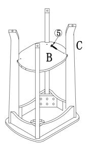
Tighten Bottom Panel (B) to the one Leg (C) using Screw (5). Place the table on the floor and check if it is stable before tightening all bolts.
