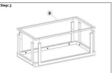
Please keep all screws loose and tighten TOGETHER after assembling.
