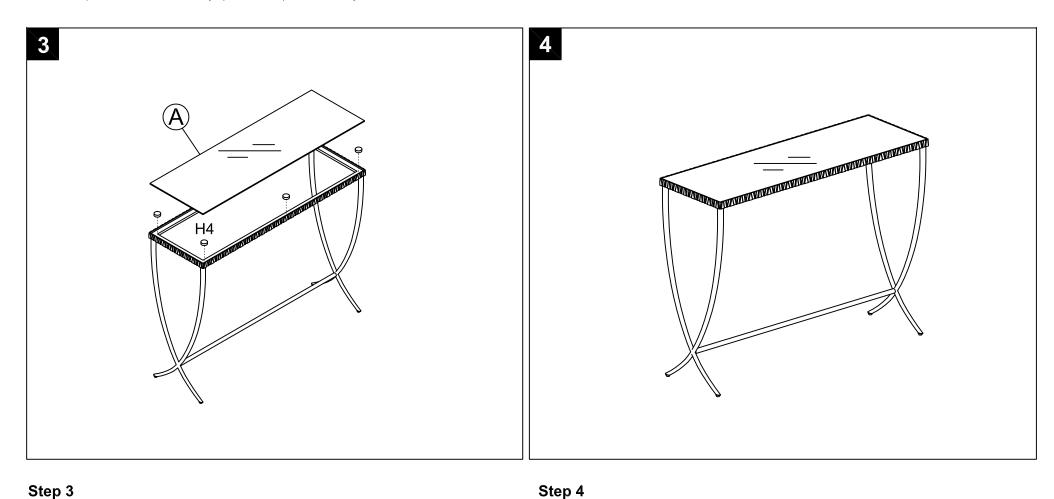
Place Transparent silicone pads (H3) on top of metal table frame before having mirror (A) placed on top.
