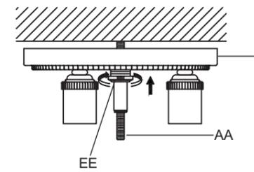
5. Place the fixture frame (B) over the nipple of mounting strip (AA), securing with previously removed finial (DD).
