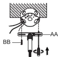
3. Strip 3/4 in. of insulation from fixture wire ends. Twist stripped ends together with pliers (not included), black to black (power), white to white (neutral). Snip ends. Wrap the ground wire from the outlet box around the green screw preassembled on the mounting strip (AA), and then connect the ground wire from the outlet box to the ground wire from the fixture.
