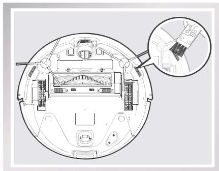
Wipe the Bumper with the brush of the Multi-Function Cleaning Tool.
