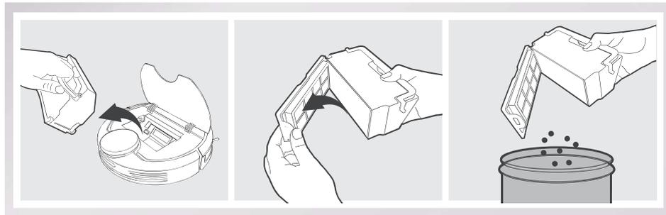
Remove the filters. Pat the High Efficiency Filter clean. Do not rinse the High Efficiency Filter under water.
