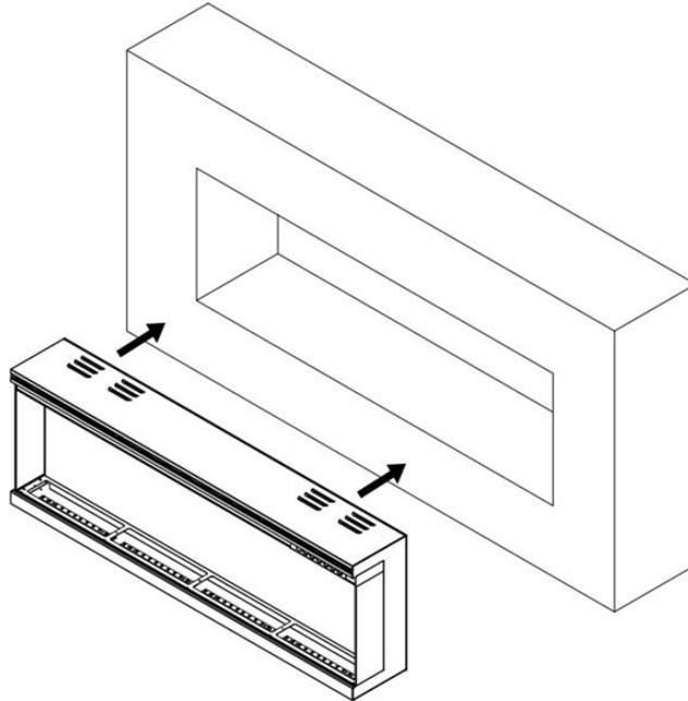
4. Once the fireplace is placed in the wall opening, secure the fireplace to the floor of the opening with 2 wood screws provided as shown below.
