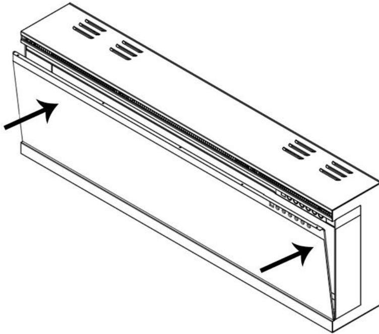
2. Reattach the screws holding the glass panel in place, as shown below.
