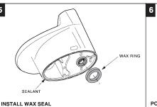
Invert toilet on floor (cushion to prevent damage), and install wax ring evenly around waste flange (horn), with tapered end of ring facing toilet. Apply a thin bead of sealant around toilet base
