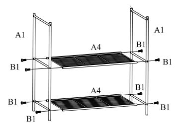
Assemble Lower Side Frames A1 to Lower Net Racks A4 using Bolts B1. Note: Please do not tighten Bolts B1 until Step 6.
