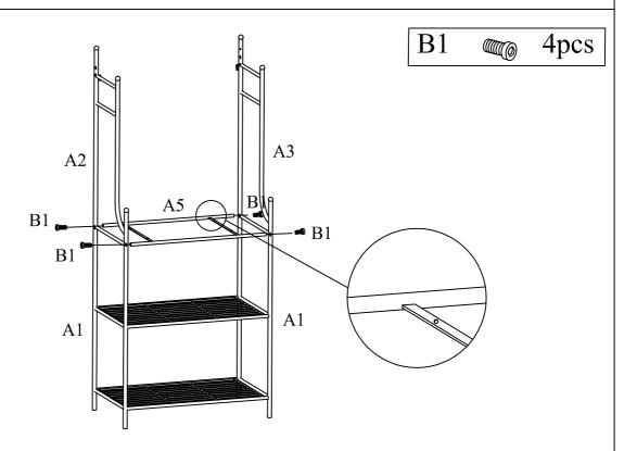
Assemble Middle Frame A5 to Side Frames A1&A2&A3 using Bolts B1. Note: Please do not tighten Bolts B1 until Step 6.
