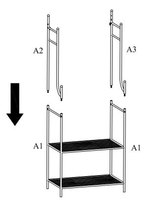
Insert Upper Side Frames A2&A3 to Lower Side Frames A1 as shown above.
