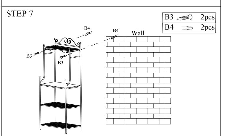
For your safety, please attach this unit to the wall by Screws B3 and Anchors B4.
