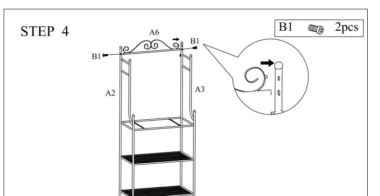
Assemble Upper Back Apron A6 to Upper Side Frames A2&A3 using Bolts B1 as shown above.
