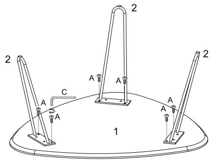
Use wrench (C), bolt (A) to secure the legs (2) to the table top (1).
