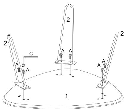
Use wrench (C), to secure legs(2) to the table top (1) with bolts (A).
