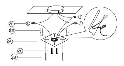
Drill two holes on the ceiling and put the plastic anchor screw(ZE) into the holes(If the wall is wood made, this step can be ignored);
