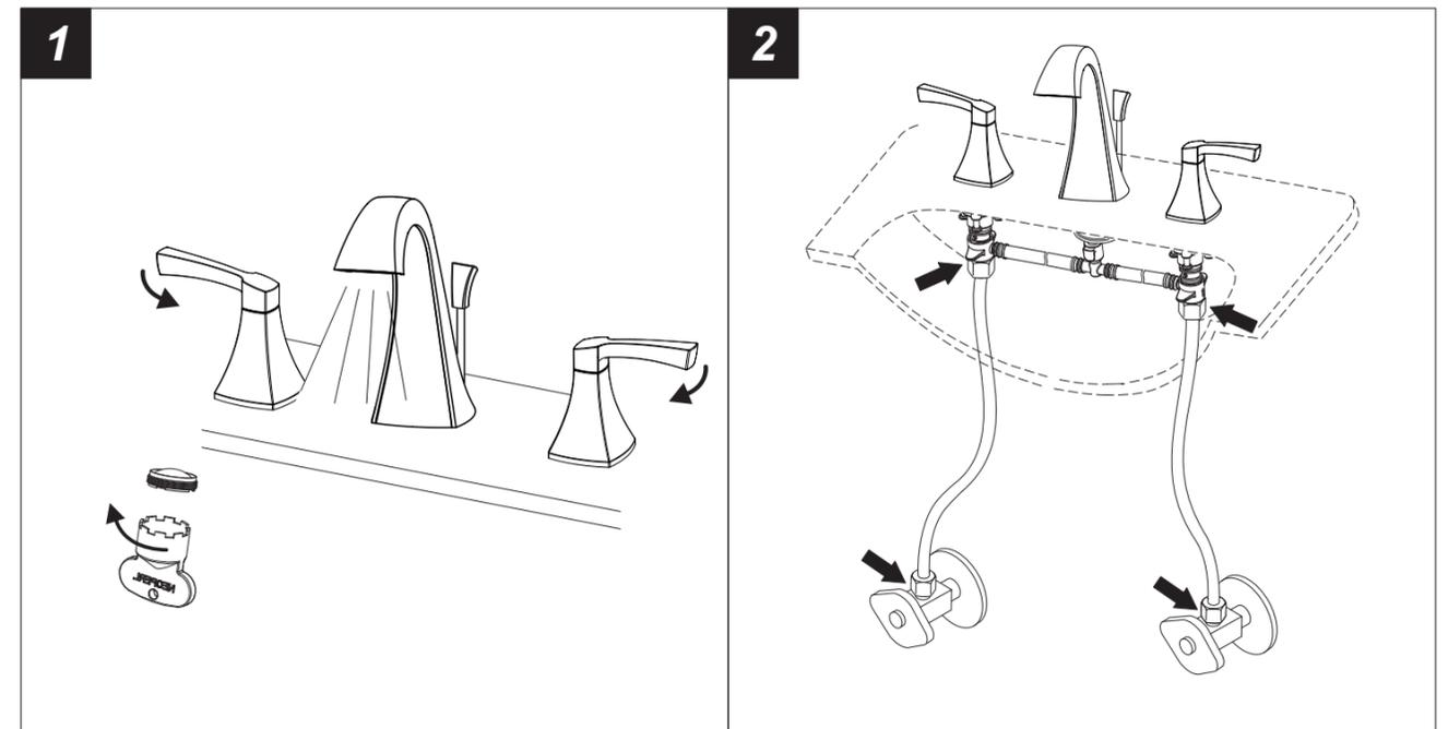
1. Remove the aerator by aerator wrench. Turn the faucet handle all the way on, turn on hot and cold water supply and flush water lines for one minute. Reinstall aerator by aerator wrench.
